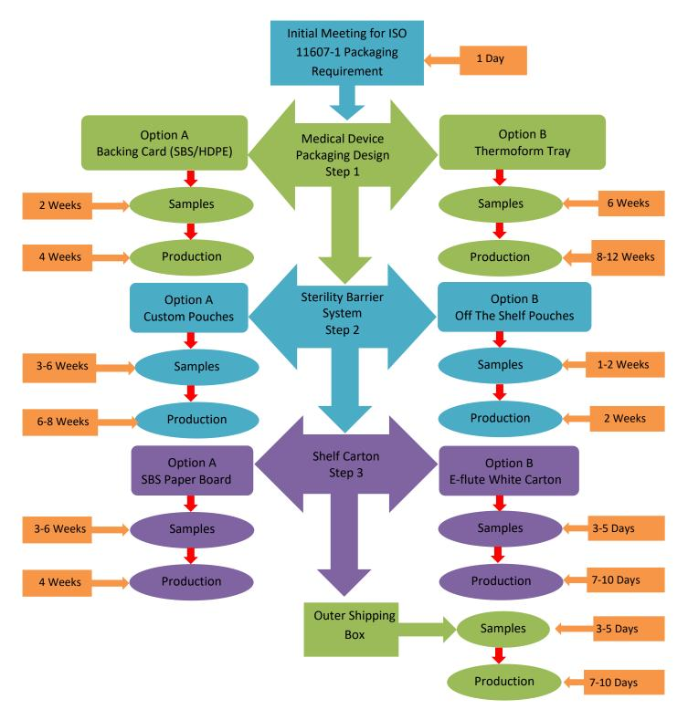
By using the above chart to plan sample testing requirement of 29 (plus three additional packaging units recommended not required), it can take four to six month for the overall process which is only the initial phase of Packaging design and getting ready for Packaging validation testing.
